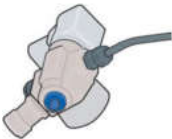
Manual shut-off valve on the foot of the cylinder valve.
