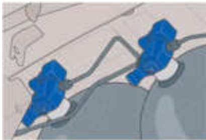
Electromagnetic shut-off valves on the gas tanks
